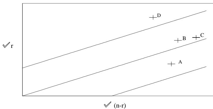
these values, the scales are contracted by multiplying them with the appropriate factor. If the factor ten is applied to both scales, the tenth scale usually drawn on the top of the BIPP chart is used to set the limits. This scale has a distance of 0.063 inches per standard deviation (0.2 inches divided by 10.)
